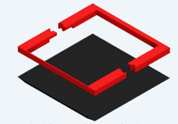
The primary method for manufacturing for this component will be Injection Moulding. As there is an internal undercut in this piece, a standard injection Moulding process won't be sufficient. The component will be manufactured in 3 sections - the base and the two internal recesses. These pieces will then be joined by adhesive bonding and a drilling operation will create the holes for the spring bearings.
