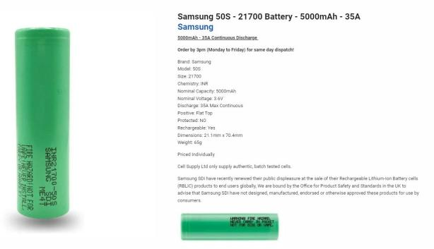
Above cell is 5Ah and has a nominal voltage of 3.6V. A target goal between 75Wh-100Wh. The configuration is 12S/13S1P. With 12S a nominal voltage of 43.2V with a power of 216Wh is produced. With 13S a nominal voltage of 46.8V with a power of 234Wh is produced. 12S is sufficient to meet power goals set
