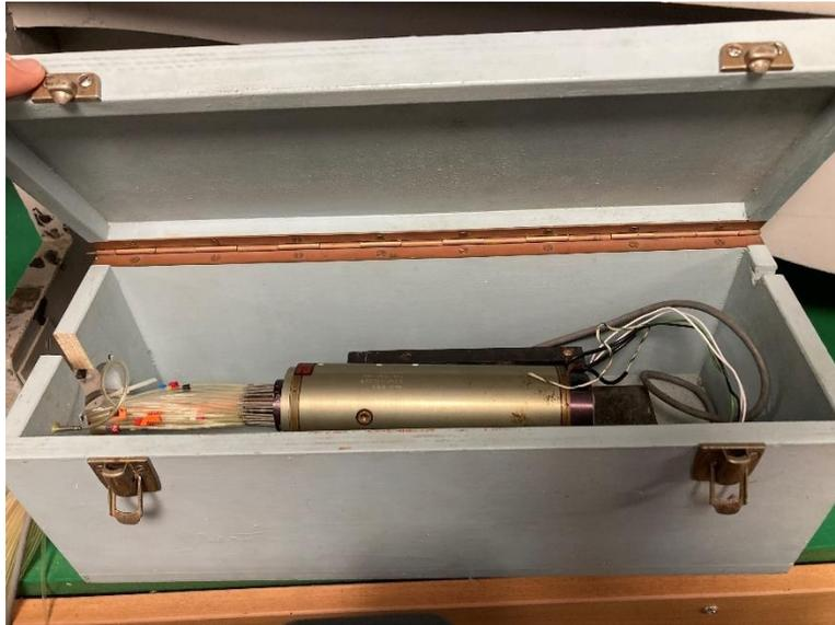
Figure 4: The pressure transducer connected to the 33 pressure taps on the aerofoil.
