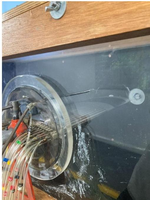
Figure 3: Image showing the 33 pressure taps on the aerofoil that are connected to a pressure transducer. The transducer outputs signals to the Scanivalve program, enabling measurements of the pressure distribution over the aerofoil.
