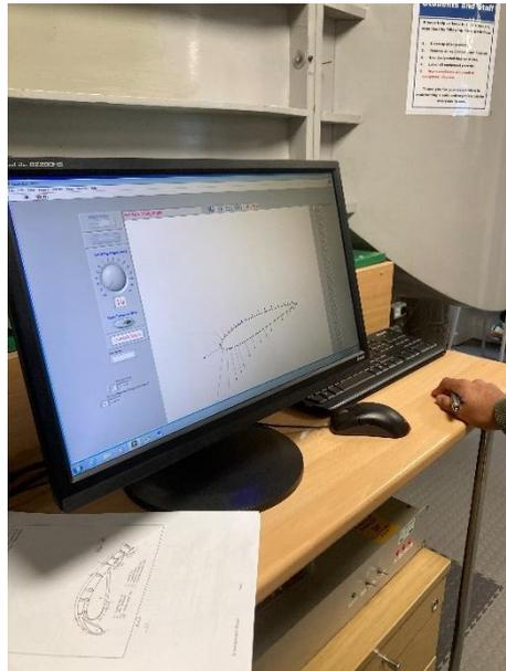
Figure 5: The Scanivalve programme receiving data from the pressure transducer. This program performed trapezoidal integration to interpolate the pressure distribution over the aerofoil from the 33 pressure taps.
